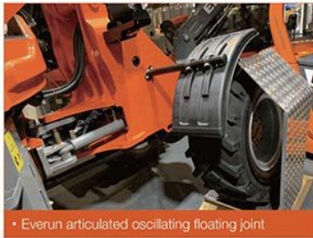
• Everun articulated oscillating floating joint
