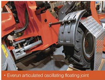
• Everun articulated oscillating floating joint
