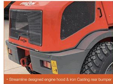
• Streamline designed engine hood & iron Casting rear bumper
