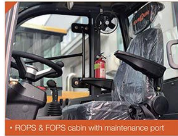
• ROPS & FOPS cabin with maintenance port
